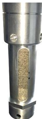
A formation with an estimated 10 Darcy permeability can be simulated by 20~40 mesh frac-sand bed.
