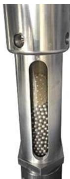
A vugular formation prone to loss circulation can be simulated by a pack of 5 mm steel beads.
