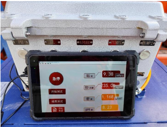
Fig 1. REALologyFAST integrated into a fracturing fluid monitoring system
