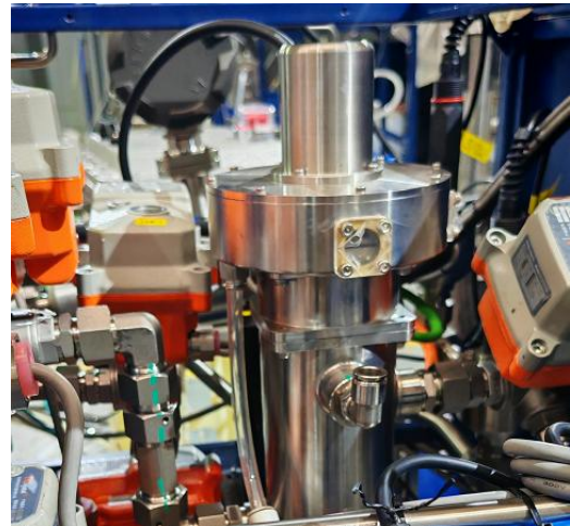
Fig 2. REALologyFAST integrated into a drilling fluid monitoring system
